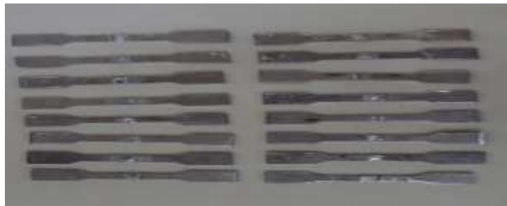
Fig 3.4 Tensile test specimen before tensile test
